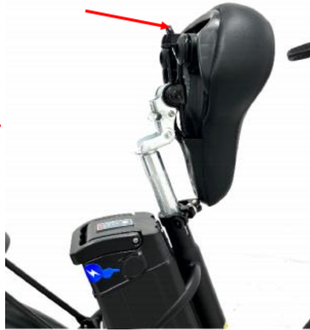
2.Hold this lever up to open the saddle.
