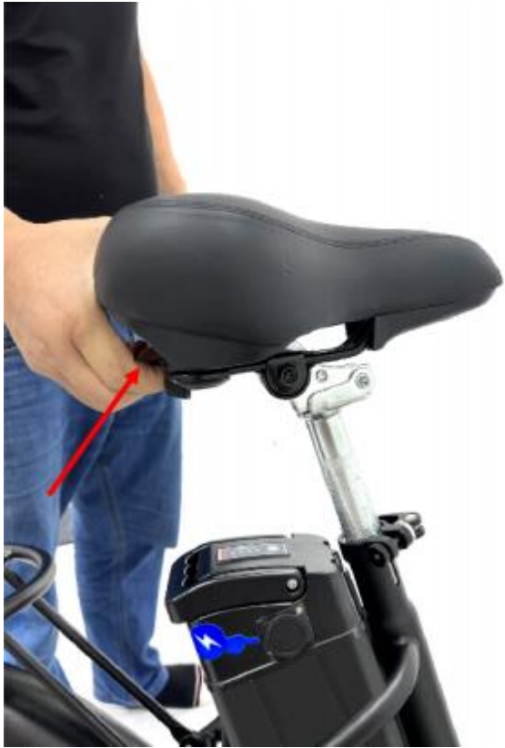
1.Pull up the flip handle at the bottom of the saddle.
